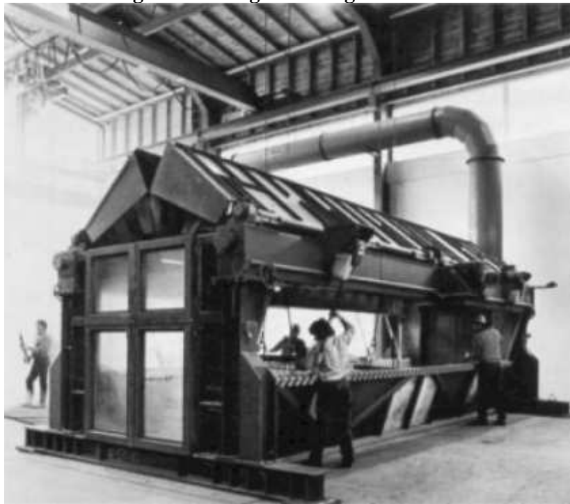
Figure 3. Zinc galvanizing enclosure 17
