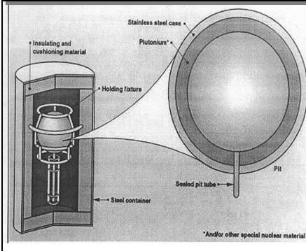
Illustration of a plutonium trigger, or "pit." Source: U.S. Department of Energy (DOE), http://www.md.doe.gov
